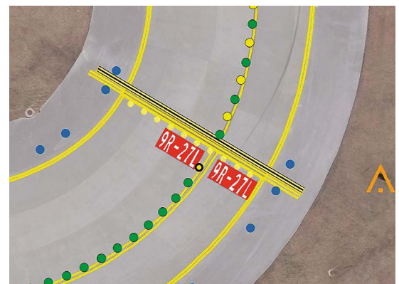
Examples of spatial data outputs required by airports that have been developed and maintained with the help of FME technology: airfield signage (top) and marking plans (bottom).
