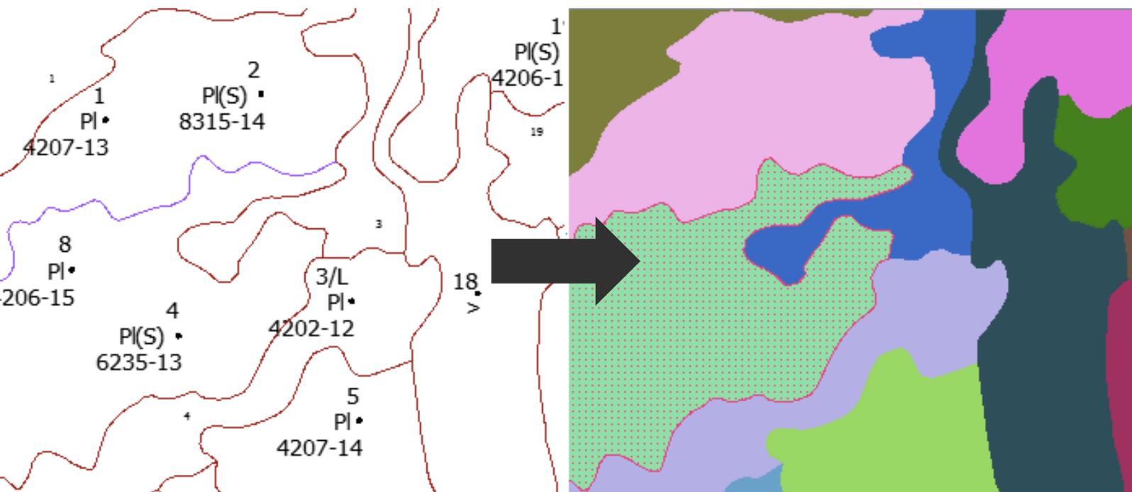
This example CAD-GIS translation has converted the linework of a design file into GIS polygons. Each polygon contains information from the CAD label points. The label can be used to get other attribute information using a database join.
